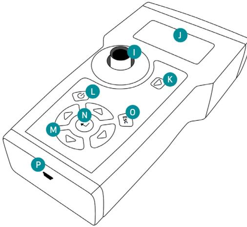
**I** Measurement chamber for iCheck Iodine reagent vials with removable metal cap (not shown)
