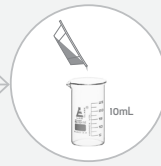
Transfer the ground FK to a beaker and dilute to a 0.4% sodium hydroxide solution. Pre-digestion with amylase may be required.
