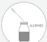
Transfer part of the FK slurry to a new flask and acidify with 0.2 M HCl
