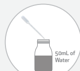
Transfer 1 mL of FK slurry to a new flask and fill up to 50 mL with water.
