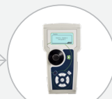
Multiply the displayed result with the corresponding dilution factor to get vitamin A concentration in FK in mg/kg .
