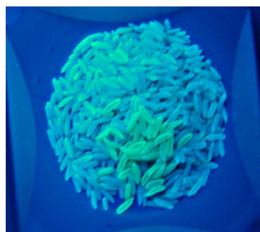
Vitamin A fortified kernels fluorescing under ultraviolet light
