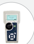
Multiply the displayed result with the corresponding dilution factor to get iron concentration in FK in mg/kg .
